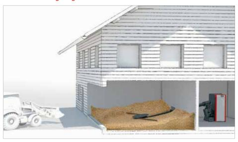
Direct filling of storage room, transport to boiler via auger
