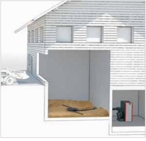
Horizontal room clearing to the boiler
