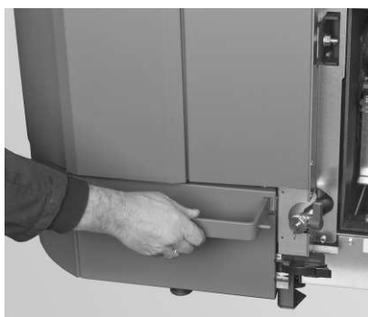
Fig. 31 Pull out the handle
