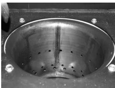
Fig. 47 Clean the secondary air holes in the burner bowl
