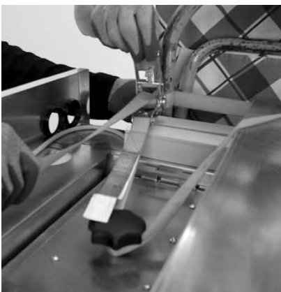
Fig. 11 Secure boiler to sack truck with ratchet strap
