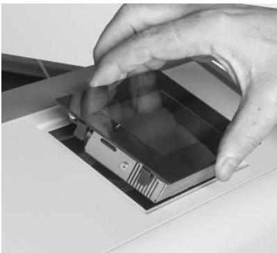
Fig. 95 Insert InfoWIN Touch into the operating panel
