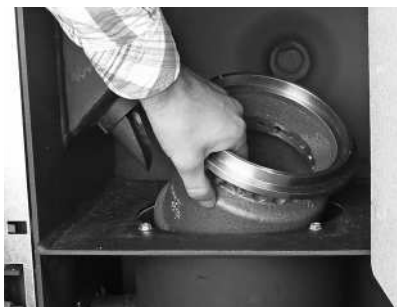
Fig. 41 Lift out bottom part of cone
