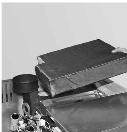
Fig. 26 Remove the insulation
