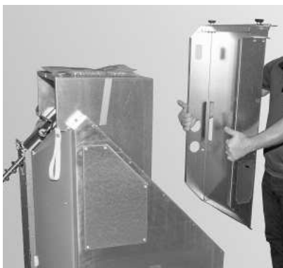
Fig. 39 Remove the foot
