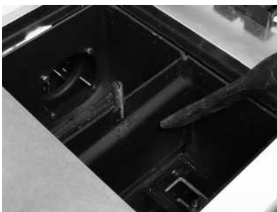
Fig. 58 Vacuum out the ash
