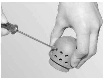
Fig. 46 Clean the primary air pin carefully
