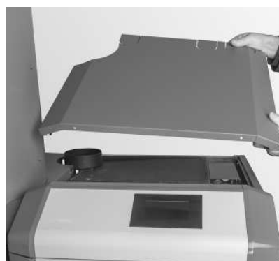
Fig. 51 Lift off the top cover
