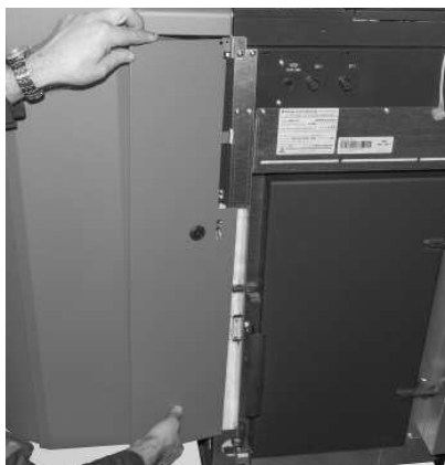
Fig. 68 Insert the front cladding
