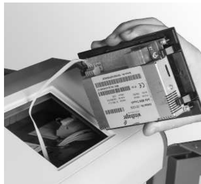
Fig. 94 Connect the InfoWIN Touch connecting cable and insert InfoWIN Touch into the operating panel (with the plug at the top)
