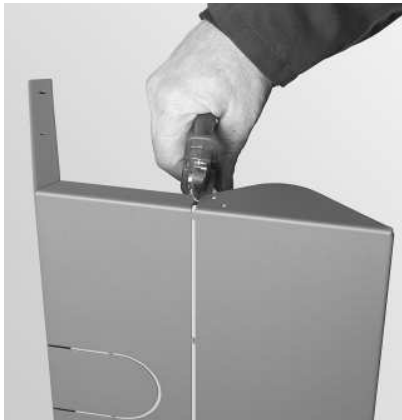
Fig. 70 Cut through web at top and bottom
