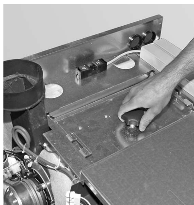
Fig. 27 Remove the screw connection
