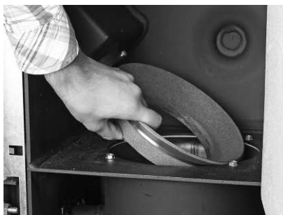
Fig. 40 Lift out top part of cone
