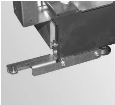
Fig. 86 Screw on the bottom door hinge
