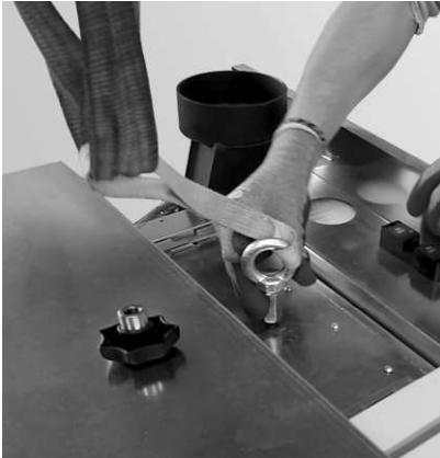
Fig. 13 Mount the eyelet (not included) for the crane hook
