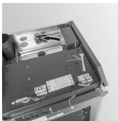
Fig. 64 Disconnect the device power plug
