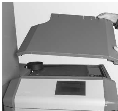
Fig. 62 Lift off the top cover
