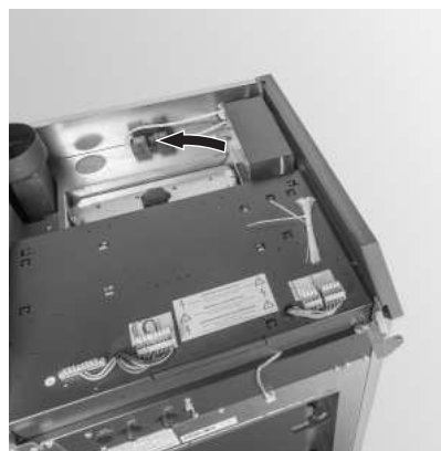
Fig. 64 Disconnect the device power plug
