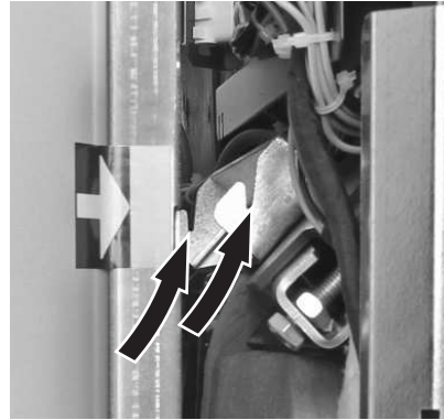
Fig. 42 Suspend the integral fuel hopper from 2 hooks, marked
