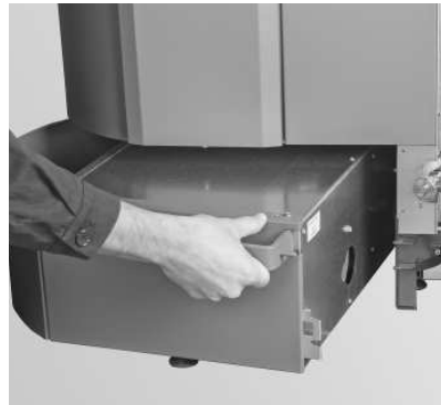
Fig. 100 Insert the ash box at a slight angle from the left and push in the ash box handle completely
