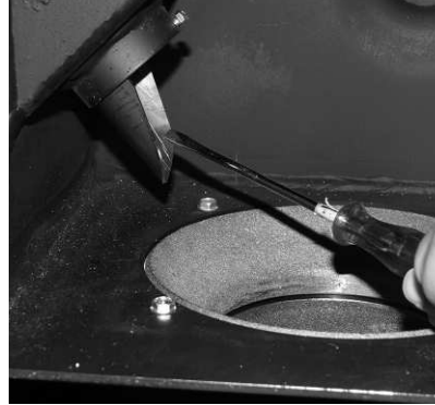
Fig. 38 Clean the down chute
