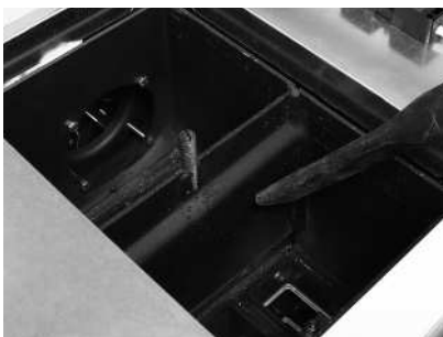
Fig. 58 Vacuum out the ash
