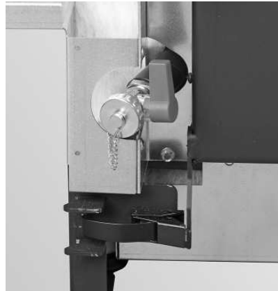
Fig. 25 Screw the drain cock (handle positioned on right) into place and re-attach the handle
