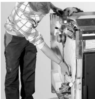
Fig. 9 Grip position for auger tube and flue outlets
