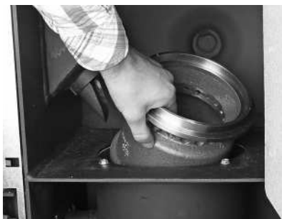
Fig. 41 Lift out bottom part of cone
