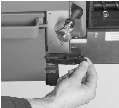
Fig. 101 Close the ash box fastener
