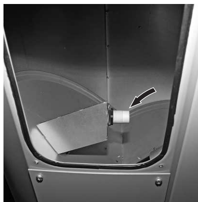
Fig. 69 Feed unit proximity switch
