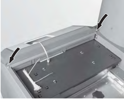
Fig. 116 Loosen the 4 screws on the operating panel
